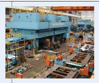
In response to needs in the U.S. auto manufacturing market, Komatsu develops fully-automatic transfer presses that deliver high-productivity features, such as fully-automated die change and the first servo-controlled transfer feeder.
