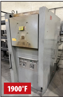
WILD BARFIELD HW1610 ELECTRIC FURNACE
