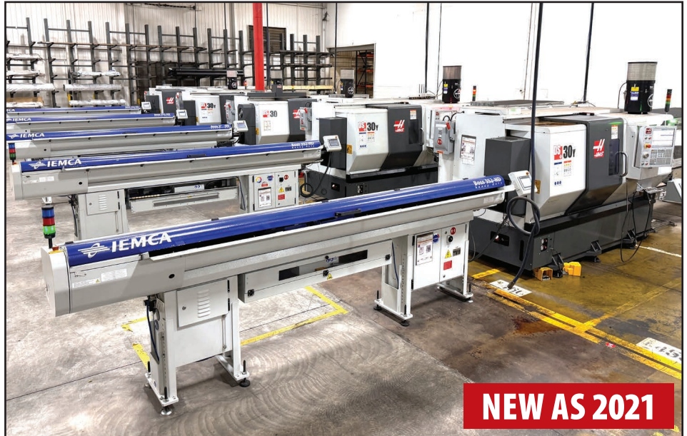
VIEW OF HAAS DS-30Y TURNING CENTERS
