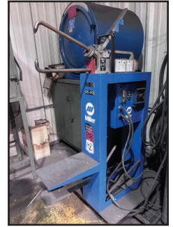
MILLER LMSW-52T SPOT WELDER
