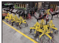
VIEW OF PIPE STANDS
