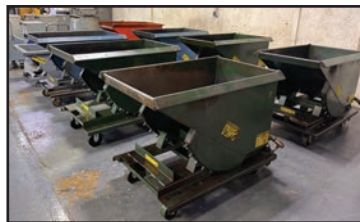
VIEW OF SELF DUMPING HOPPERS
