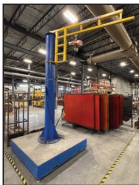
2022 FRONTENAC 500 LB. PORTABLE FREE-STANDING JIB CRANE
