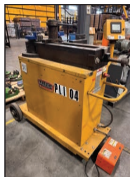
2015 BAILEIGH/RUSCH M325 PROGRAMMABLE ROTARY DRAW BENDER
