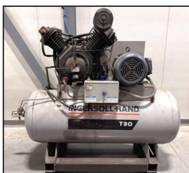
INGERSOLL RAND 15 HP AIR COMPRESSOR
