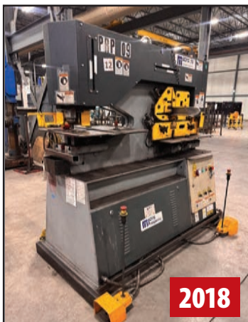
MACRO PROSPERITY 70 TON HYDRAULIC IRONWORKER
